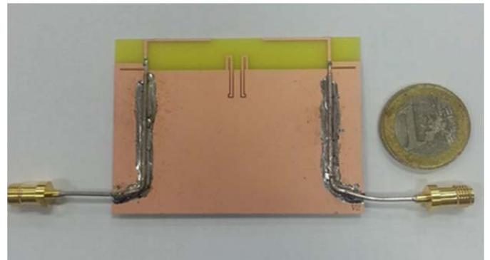
Fig. 7. Configuration of the fabricated radio frequency choke (RFC) in the MIMO antenna configuration.
