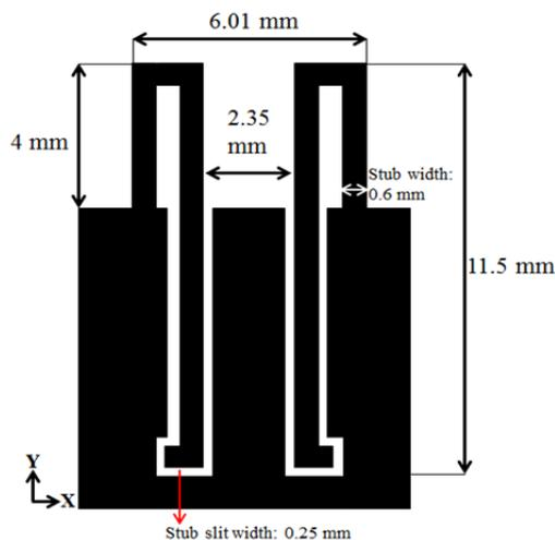
Fig. 1. Configuration of the proposed radio frequency choke.
