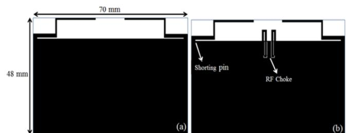
Fig. 3. Overall MIMO configuration: (a) without the radio frequency choke and (b) with the radio frequency choke.
