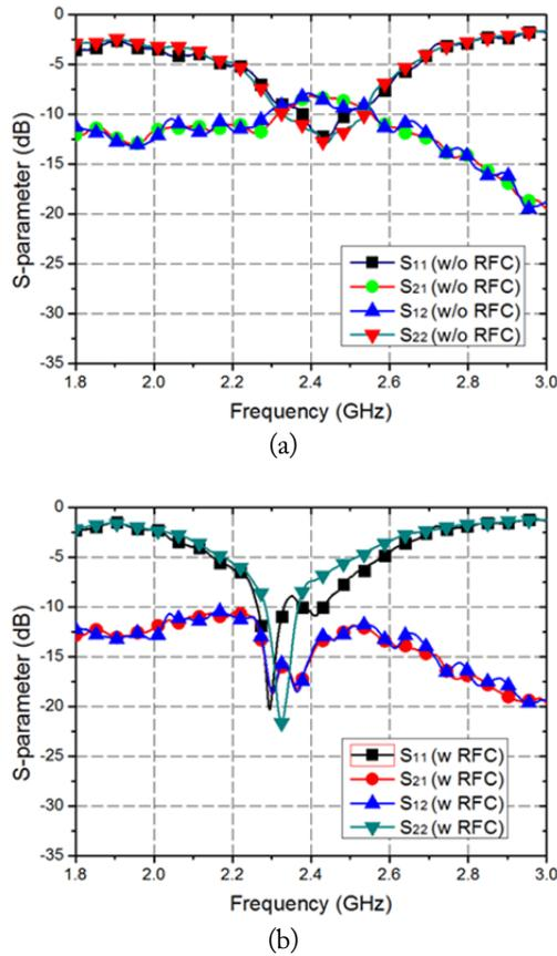
Fig. 8. Measured  $S$ -parameter characteristics (a) without the radio frequency choke (RFC) and (b) with the RFC.
