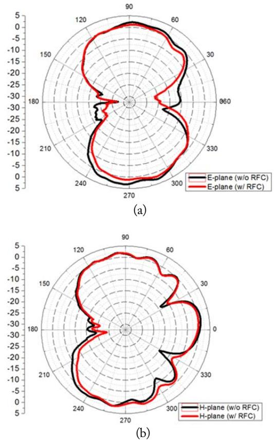
Fig. 9. Comparison of measured radiation patterns with and without the radio frequency choke (RFC). (a) E-plane and (b) H-plane.
