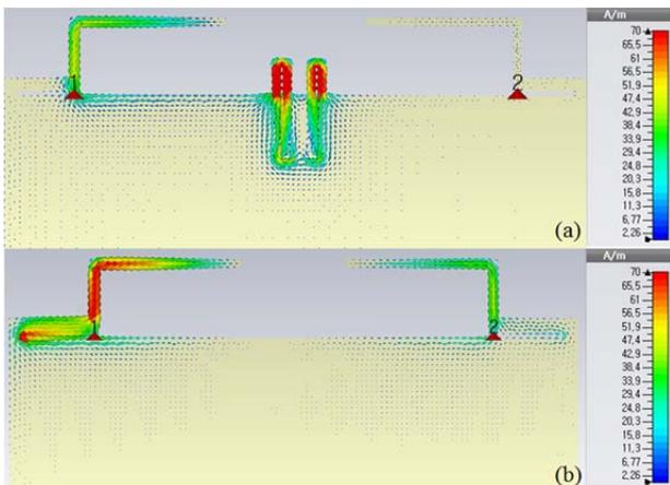
Fig. 5. Simulated current distribution (a) with the radio frequency choke (RFC) and (b) without the RFC.
