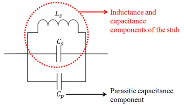
Fig. 2. Equivalent model of stub structure.
