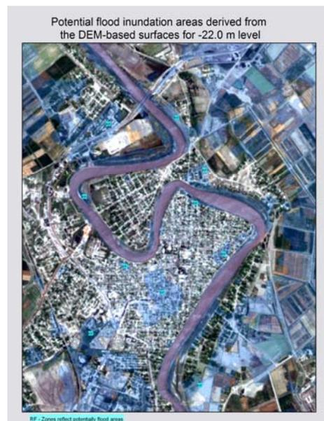
Fig. 5. Forecasting of the potentially flood inundation areas
